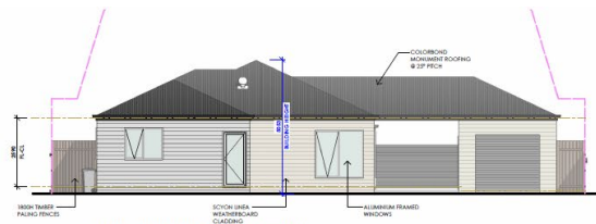
UNIT 2 ELEVATION C - (SOUTH)
